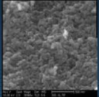
Nanoparticles compose a lightweight biocompatible material for bone implants. *Groza, 0523063.*
