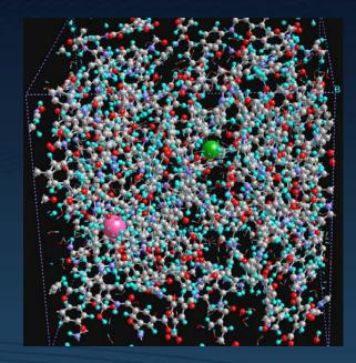
Advanced water purification and desalinization begins with understanding of how ions in water interact with purification membranes. This dynamic computer simulation shows sodium (pink) and chlorine (green) ions inside a polyamide membrane. *Shannon, 0120978.*
