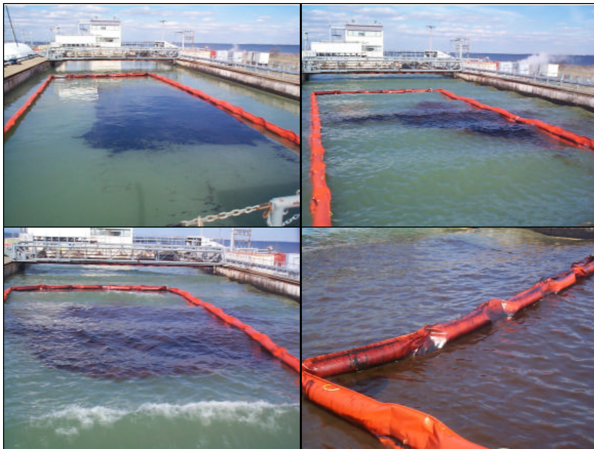
Figure 19. Photos from Test #8:10% Evaporated ANS with Corexit 9527 at 1:48 DOR
