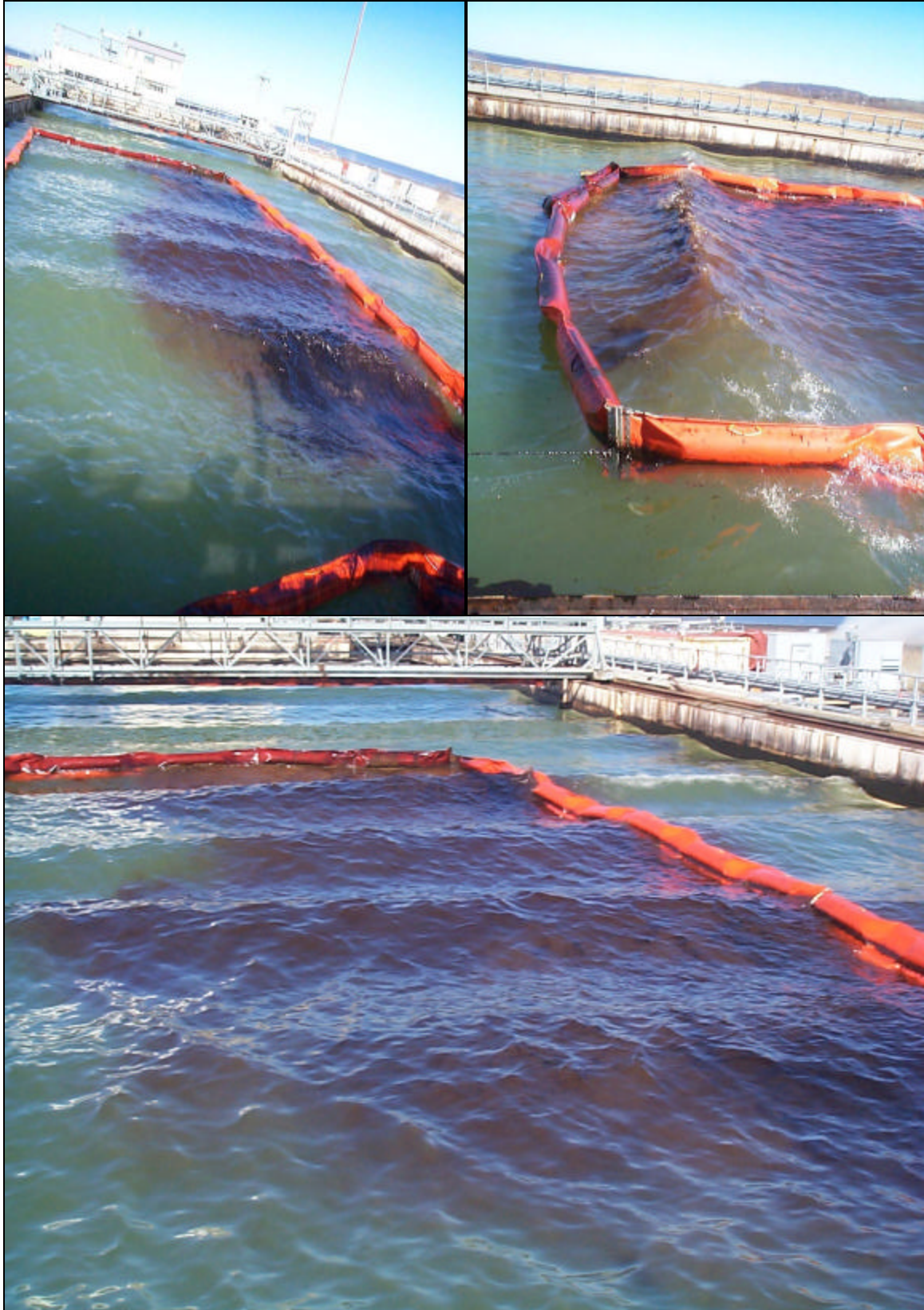
Figure 21. Photos from Test #4: Fresh ANS with Corexit 9500 at 1:34 DOR
