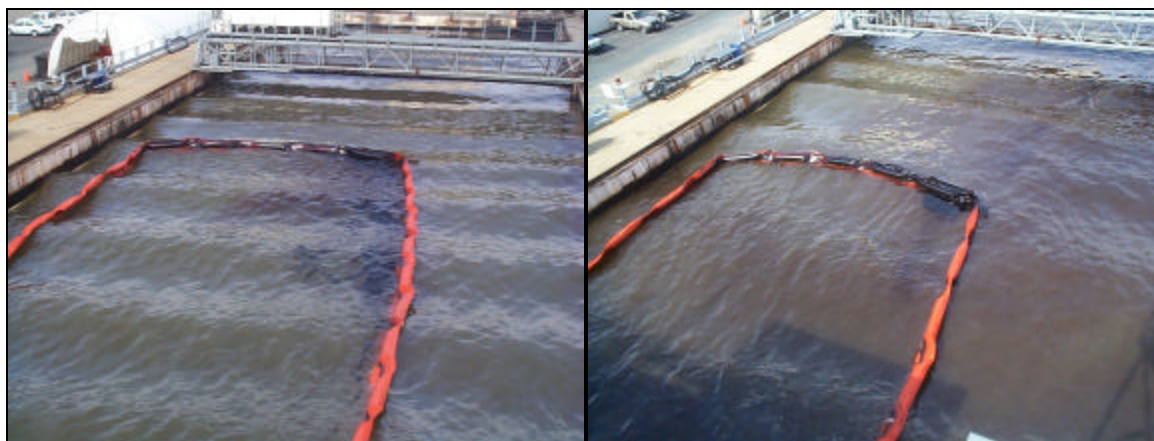
Figure 23. Photos from Test #12: 20% Evaporated ANS with Corexit 9500 at 1:38 DOR
