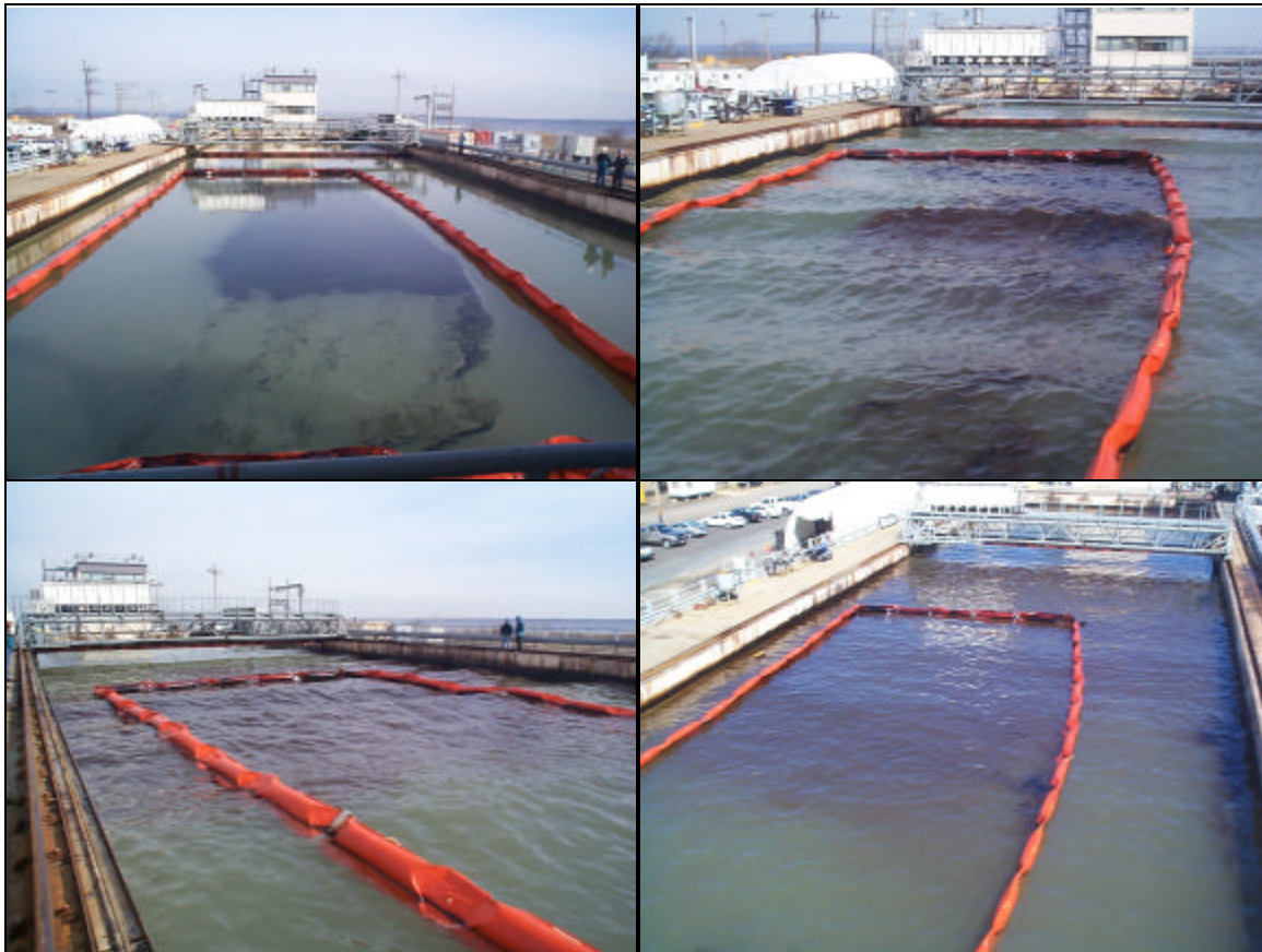
Figure 18. Photos from Test #9: Fresh ANS Treated with Corexit 9527 at 1:32 DOR
