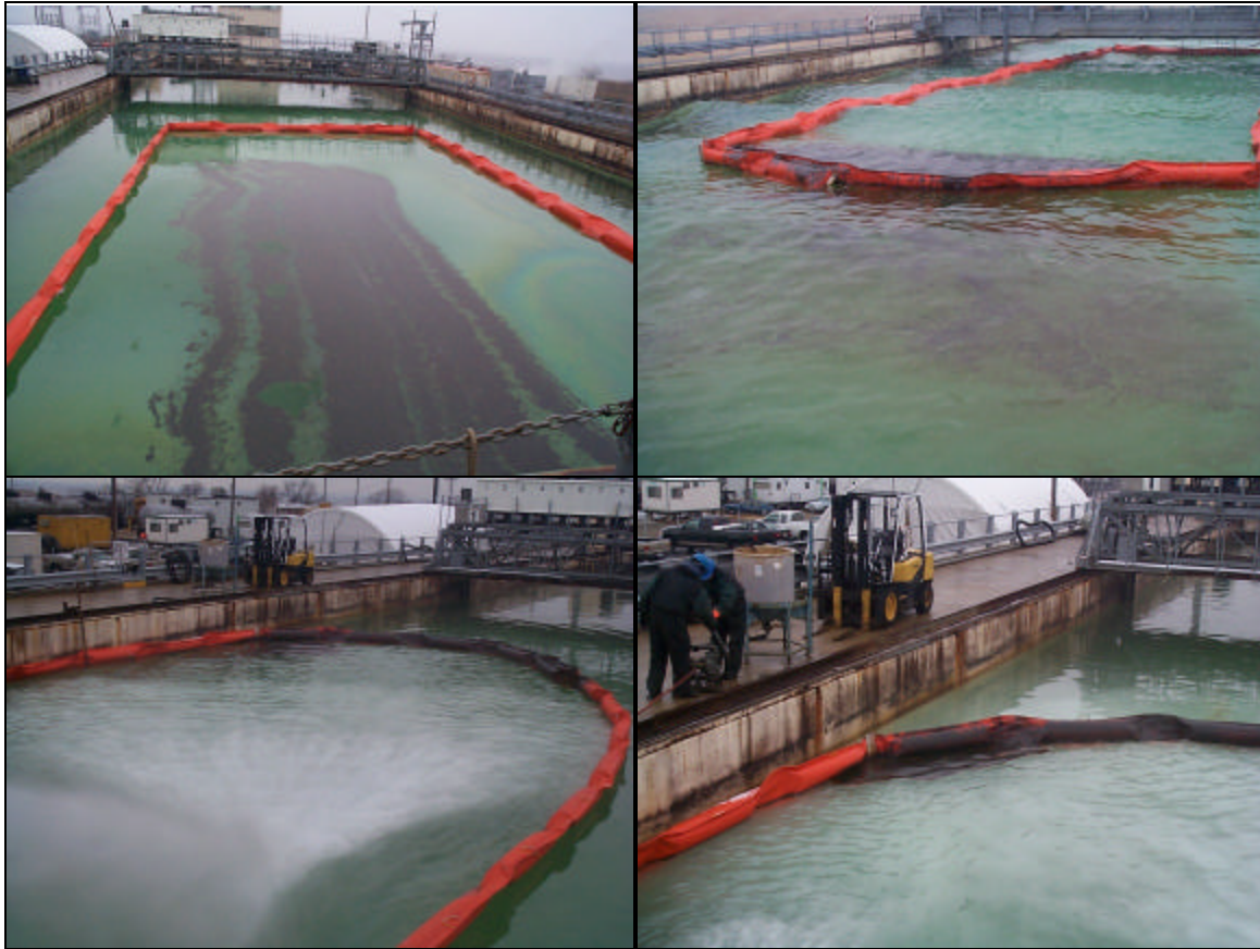
Figure 12. Photo Sequence for Hibernia Crude Oil Control Test
