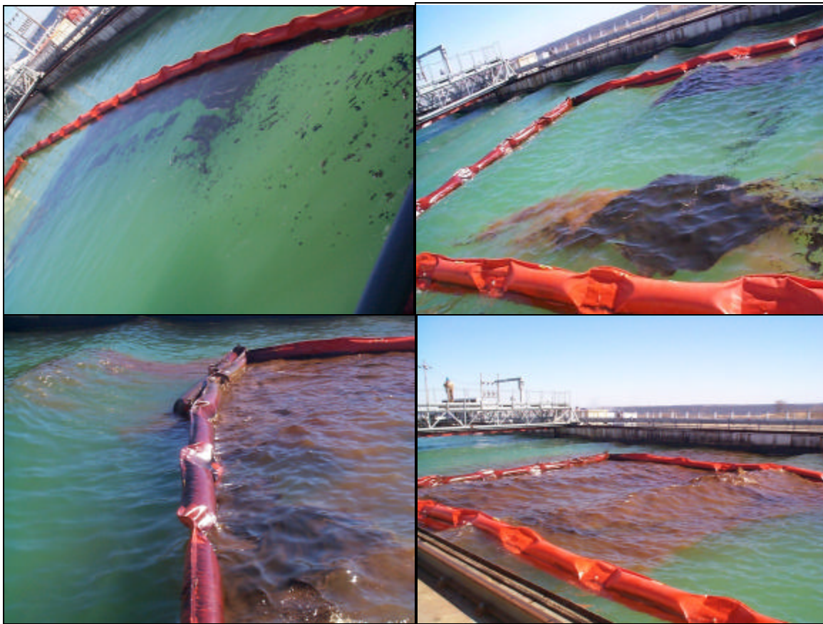
Figure 14. Photo Sequence for 7.5% Evaporated Hibernia Crude & Corexit 9500 at 1:38 DOR
