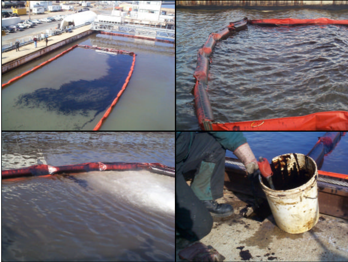
Figure 20. Photos from Test #10: 20% Evaporated ANS with Corexit 9527 at 1:44 DOR
