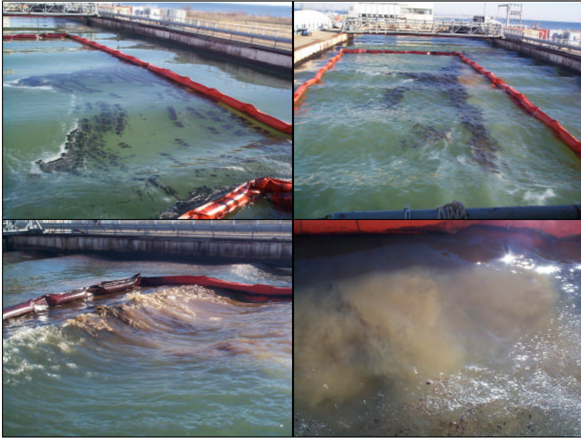
Figure 15. Photo Sequence for 10.3 % Evaporated Hibernia Crude & Corexit 9500 at 1:14 DOR
