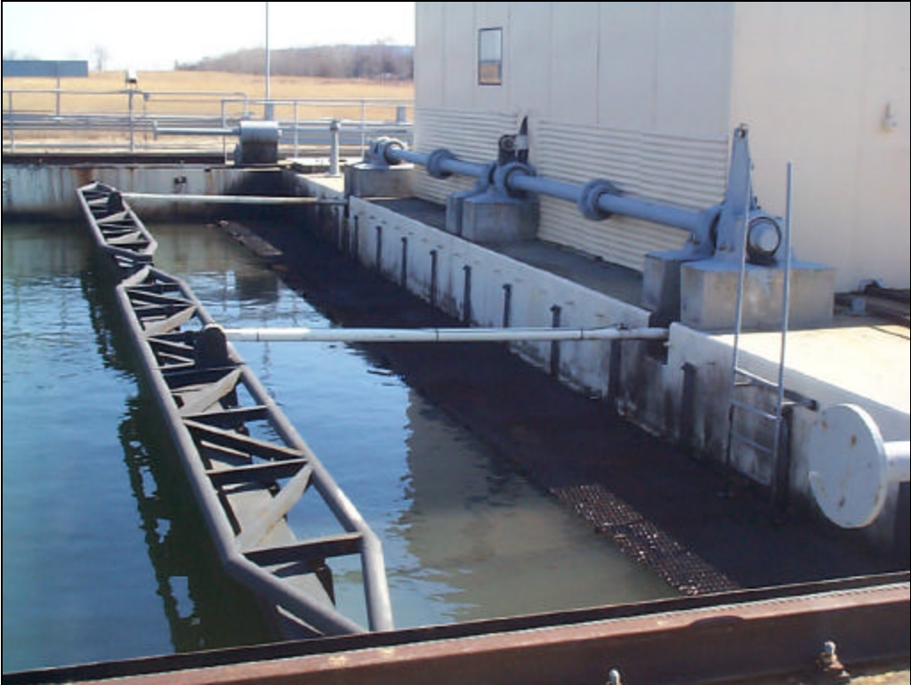
Figure 2. Ohmsett Tank Wave Paddle System
