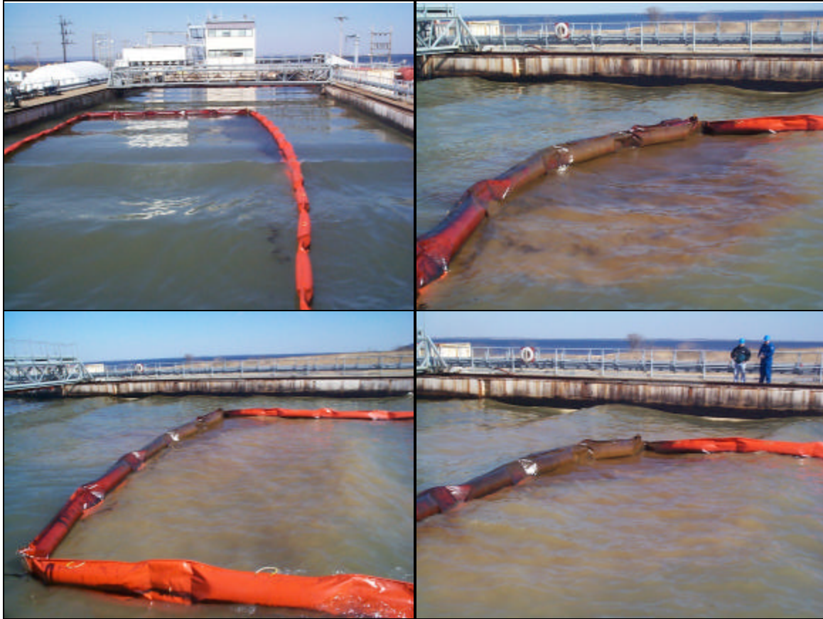
Figure 16. Photo Sequence for Hot, Fresh Hibernia Crude & Corexit 9500 at 1:14 DOR
