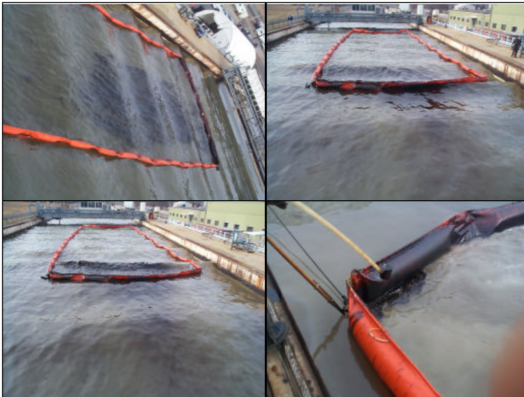
Figure 22. Photos from Test #11: Fresh ANS with Corexit 9500 at 1:81 DOR
