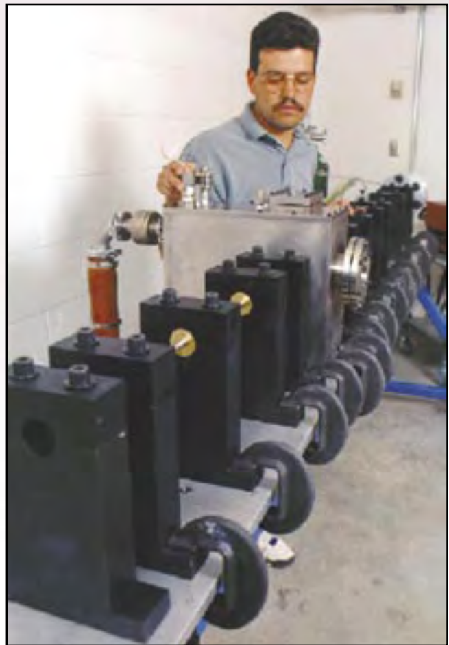
Split-Hopkinson Pressure Bar used for testing polymers and high explosives. The apparatus measures high strain rates by transmitting well-defined compressive waves to samples.
