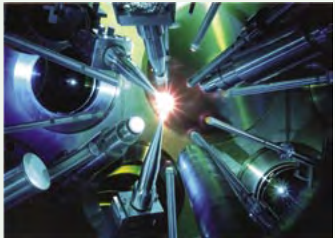
The OMEGA laser at the University of Rochester's Laboratory for Laser Energetics focuses 60 beams of laser energy onto a target (23 kJ in 1 ns). This inside view of the vacuum vessel during a shot shows the capsule (small bright reddish object) and the snouts of various diagnostics (e.g., x-ray and visible cameras).
