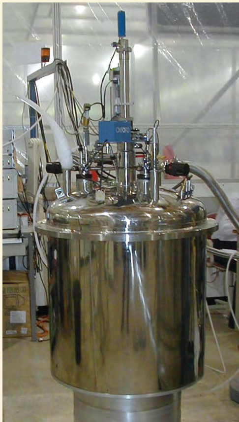
During the 2002 run cycle at the Lujan Center, the newly commissioned 11-T superconducting magnet provided users with the first results of an intensity image (reflection) of neutron data collected from an antiferromagnetic material on the new Asterix instrument.
