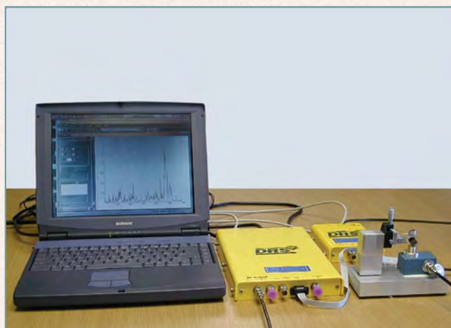
The RUS system developed by Migliori's team was commercialized by Dynamic Resonance Systems, Inc. The test jig at the right of the photograph is shown with a cubic graphite specimen mounted between the two transducers. Software to control the system and process the data is provided as part of the package.
