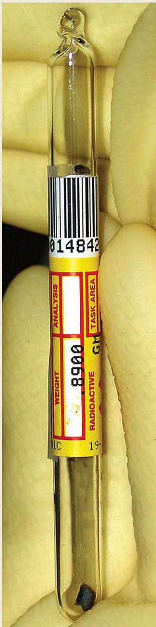
Evacuated glass ampoule containing a 1-g piece of high-purity ^{239}\text{Pu} metal that will eventually be certified by the NBL as Plutonium Metal Certified Reference Material.
