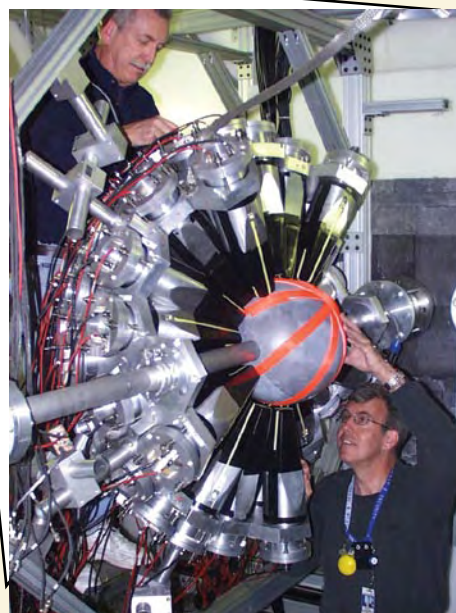
DANCE is a new gamma-ray detector at the Lujan Center. It consists of 160 BaF 2 scintillation detectors mounted as a sphere to detect as much gamma radiation as possible from a central target sample (some is lost through beam entrance and exit holes). The large photo shows the outside of the DANCE flight path; the detector is inside the large white area. The inset shows the DANCE array, split open for access. The individual BaF 2 crystals are visible, each covered with black light-tight shielding.
