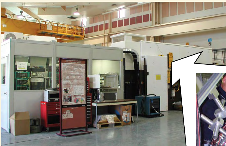
DANCE is a new gamma-ray detector at the Lujan Center. It consists of 160 BaF 2 scintillation detectors mounted as a sphere to detect as much gamma radiation as possible from a central target sample (some is lost through beam entrance and exit holes). The large photo shows the outside of the DANCE flight path; the detector is inside the large white area. The inset shows the DANCE array, split open for access. The individual BaF 2 crystals are visible, each covered with black light-tight shielding.
