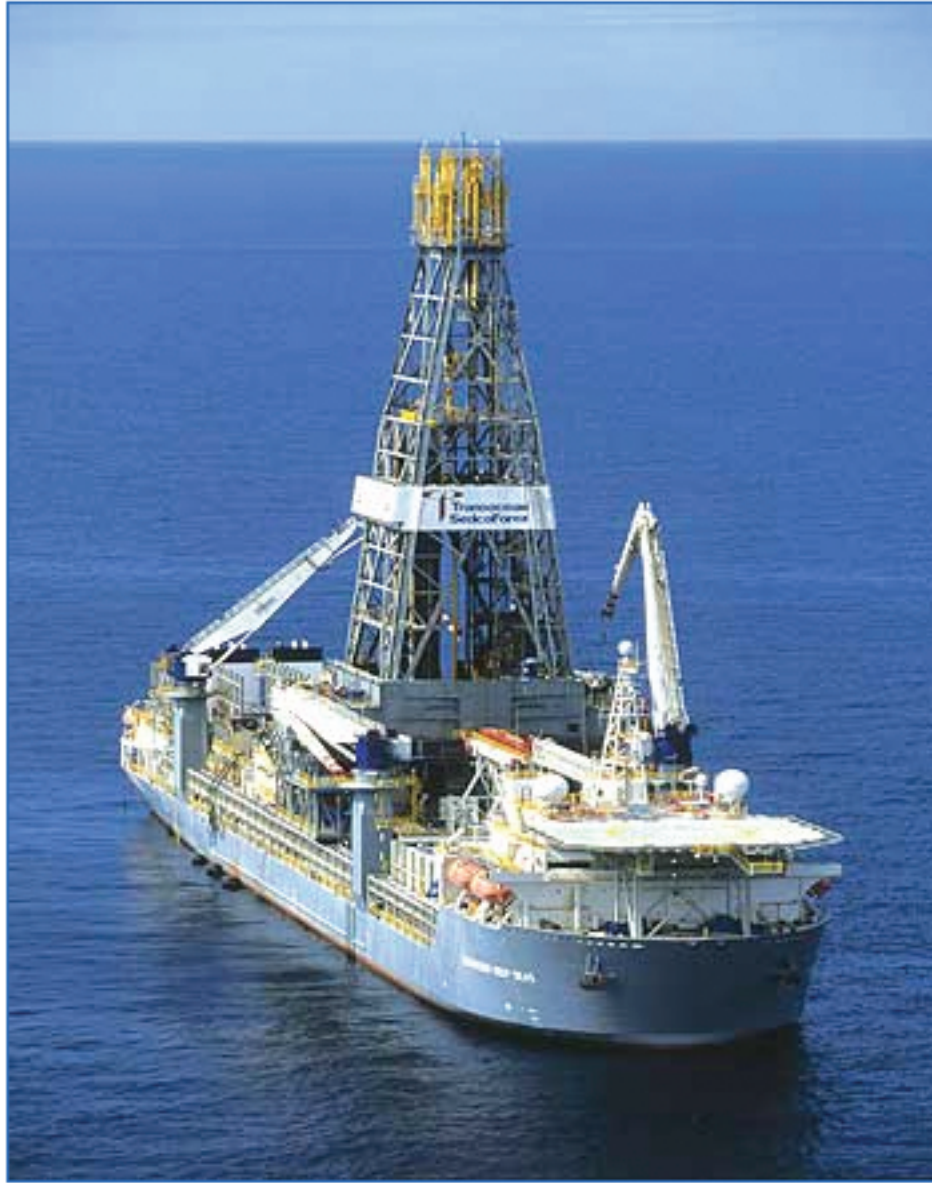
LANL's industry partner, Chevron Texaco, and its partner, Transocean Inc., achieved an industry record when Transocean's drillship, Discoverer Deep Seas, used LANL technology to drill Tonga, the deepest well ever drilled in the Gulf of Mexico, at a total vertical depth of 31,824 feet.
