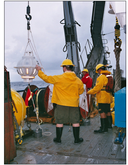
Deployment of an inverted echo sounder (IES) mooring to obtain profiles of temperature, salinity, and specific volume anomaly.
