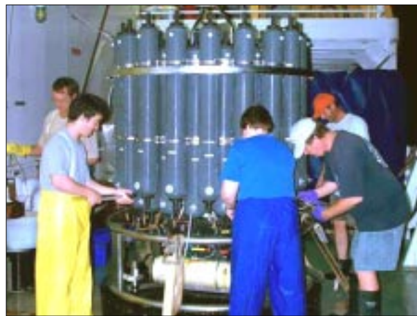
Scientists collect water samples throughout the night using a conductivity-temperature-depth (CTD) instrument.
