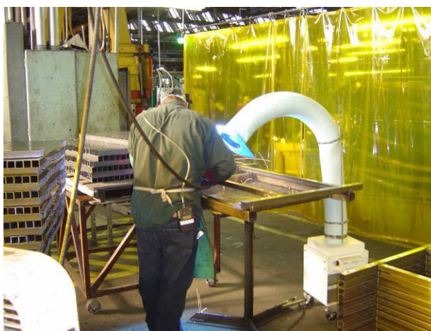
Figure 3. Welder using fume extractor.
