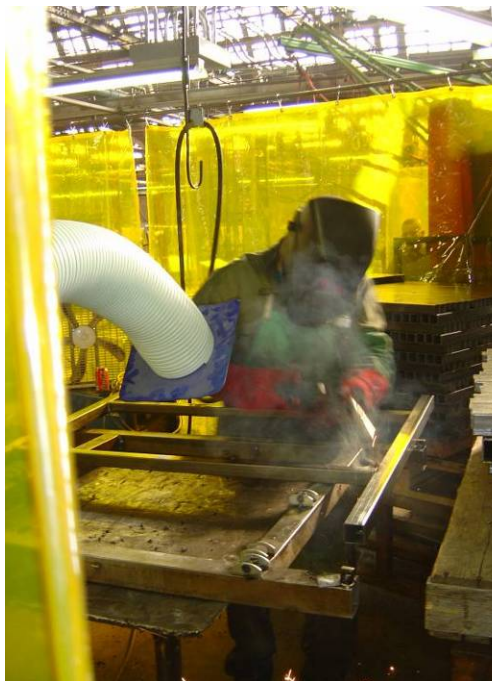
Figure 12. MIG welder leaning over previously welded area.
