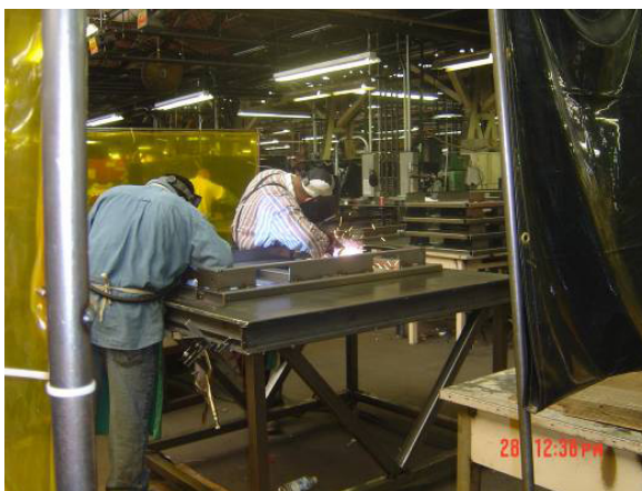
Figure 13. Two welders working on the same table without a welding curtain between them.
