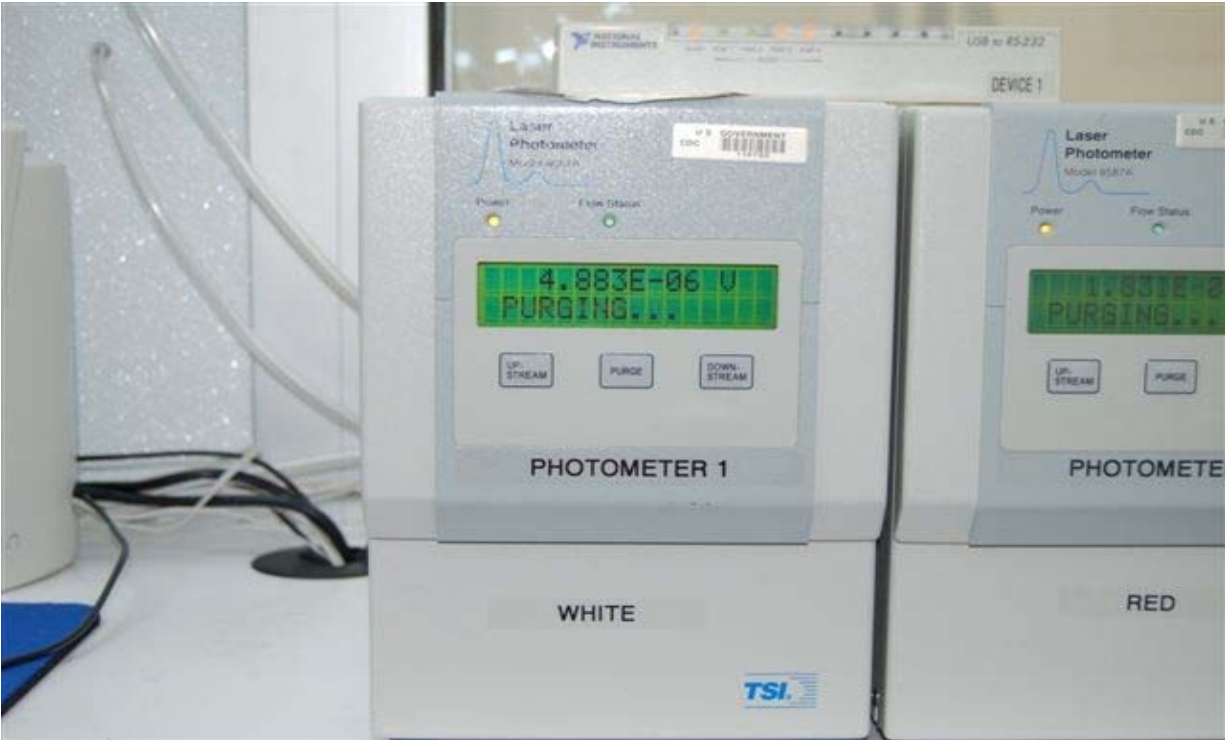
Figure 1: Laser Photometer, Model 8587A
