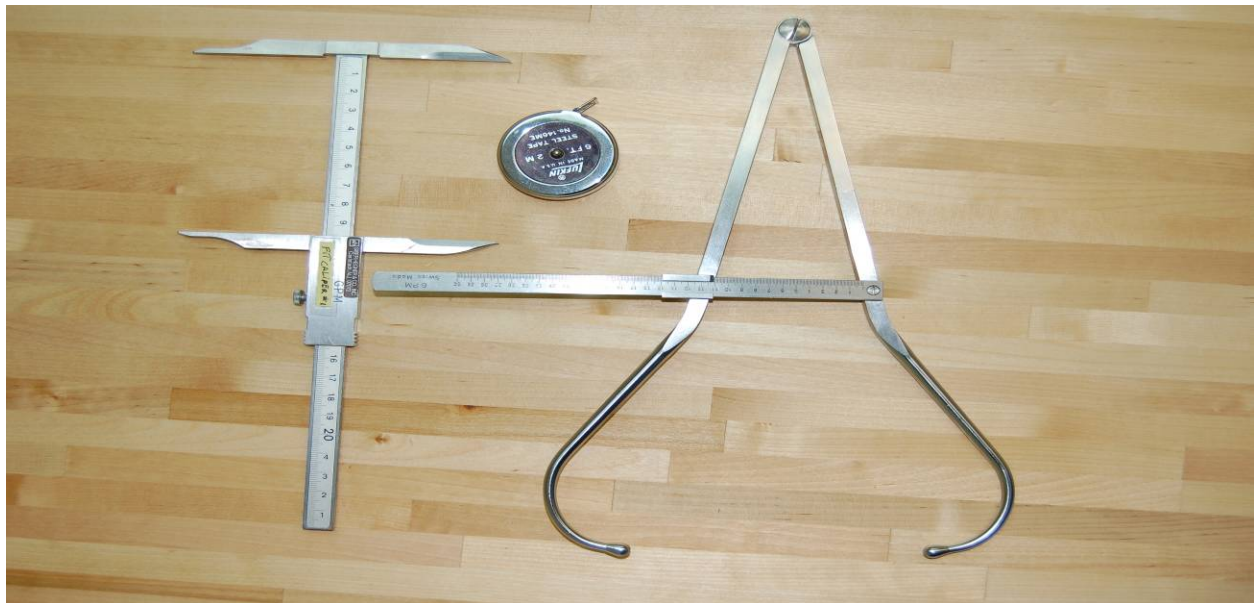
Figure 6: Facial Size Measurement Calipers
