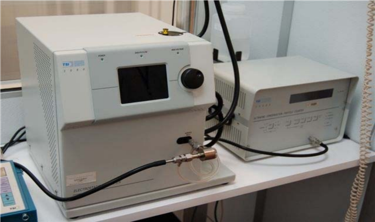
Figure 4: Scanning Mobility Particle Sizer
