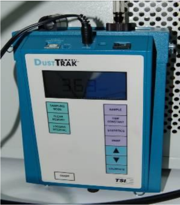
Figure 3: Dustrack Aerosol Monitor
