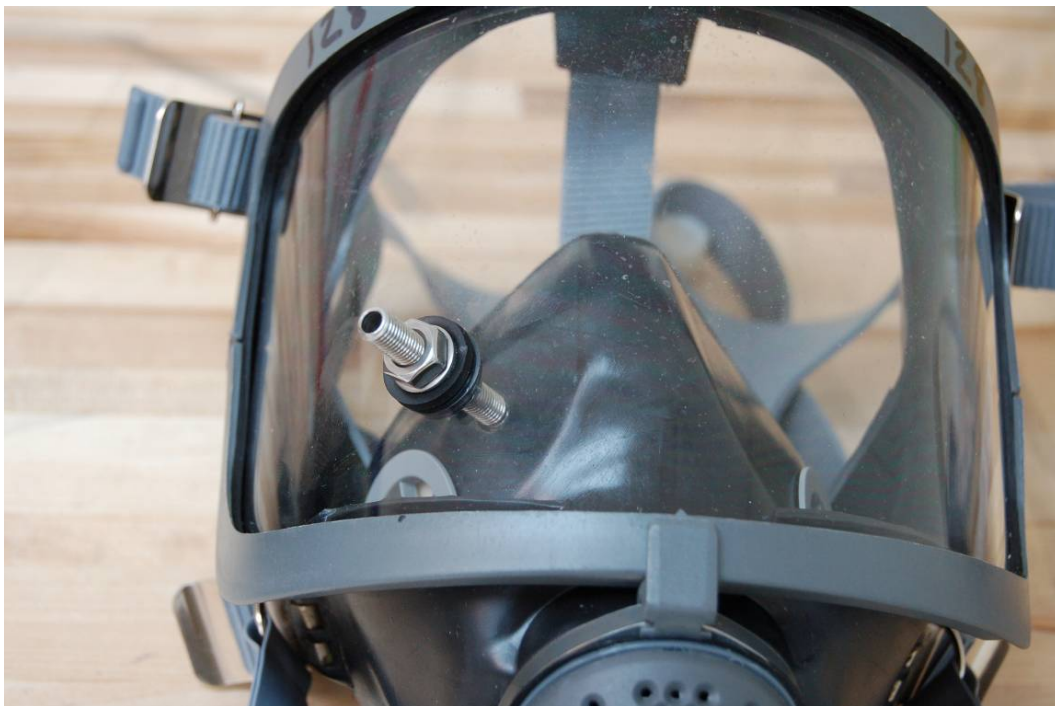
Figure 8: Exterior View of a Probed Sample Respirator
