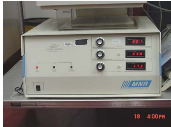
Picture 5: Flow-Temperature-Humidity Control System
