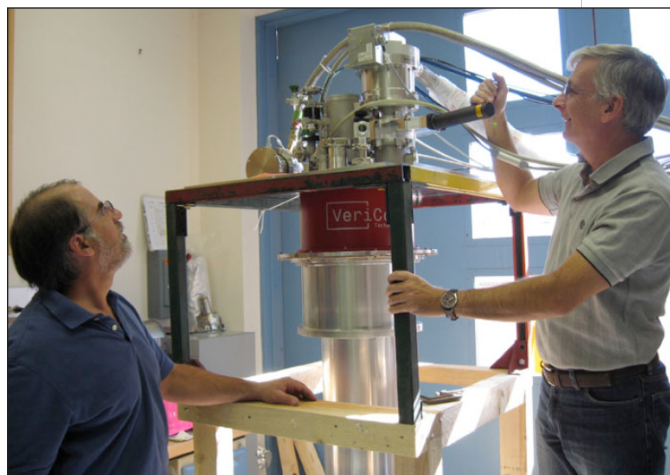
Frans Trouw (right), leader of the Lujan Center cryogenics team, and Alan Shapiro (both of LANSCE-LC), examine the new dilution refrigerator recently commissioned at the Lujan Neutron Scattering Center.
