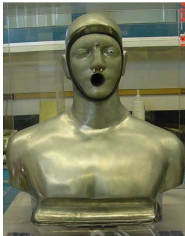
Picture 1: Head/Upper Torso Manikin, SMARTMAN
