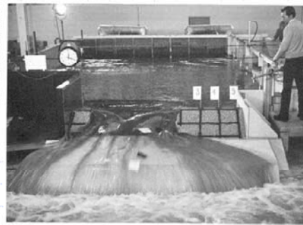
20 The lateral erosion rate was determined by timing the erosion between flags. P801-D80952
