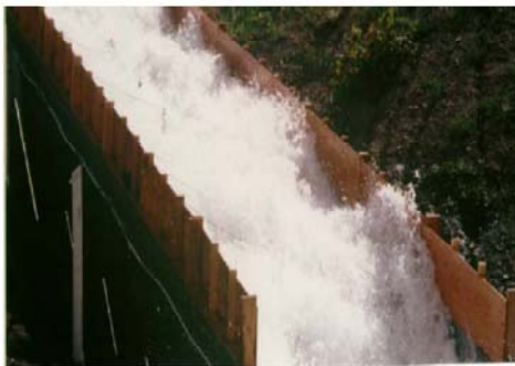
Figure 49: Large plumes of water (1995) ( Q=2.12 \text{ m}^3/\text{s} )
