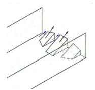
Figure 17. Dentates at the End of Chute
