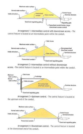
Figure 3 – Various Locations for Control Structures.
