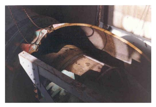
**Photo 4** - Failed needle valve.
