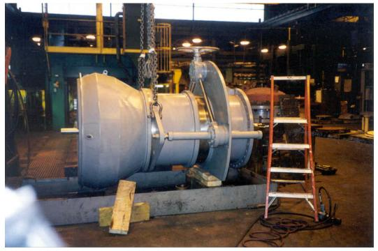
Photo 3 Fixed-Cone Valve with a Hood
