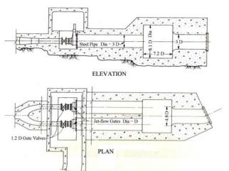
Figure 12. A sudden Enlargement in a Pipeline with Jet Flow Gates
