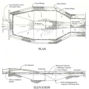
Figure 18. Plunge Pool in Connection with a Flip-Bucket
