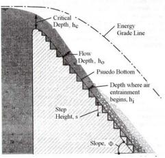
Figure 5. Stepped Spillway
