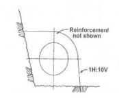
Figure 2 – Conduit Cast Against Excavated Rock
