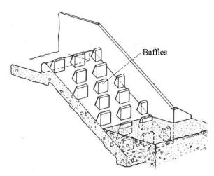
Figure 4. Baffled Apron Drop
