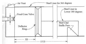
Figure 8. Fixed-cone valve installation
