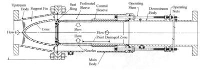
Figure 10. Orifice valve
