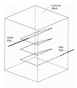
Figure 15. Elbow Energy Dissipator
