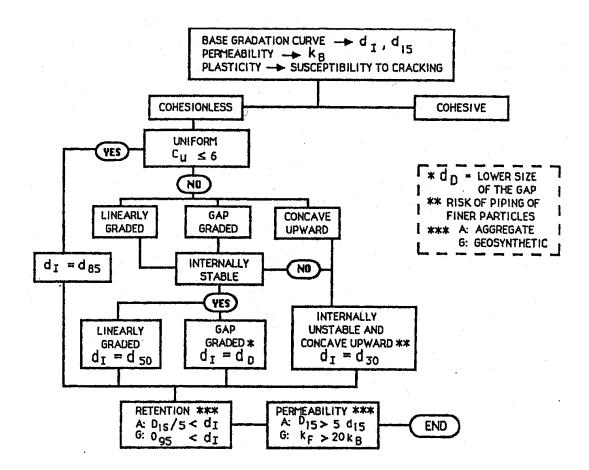
Figure 5 Lafleur et al (1993) method for the design of conventional and geotextile filters
