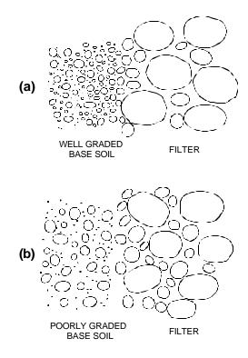
Figure 3 Filtering and self filtering concepts, (a) well graded base soil (b) gap graded, or concave graded soil, deficient in medium sized particles.
