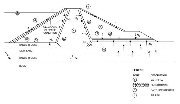
Figure 2 Flow conditions acting on filters P = Flow parallel to interface; N1 = flow normal to interface, high gradient conditions; N2 = flow normal to interface, low gradient conditions.
