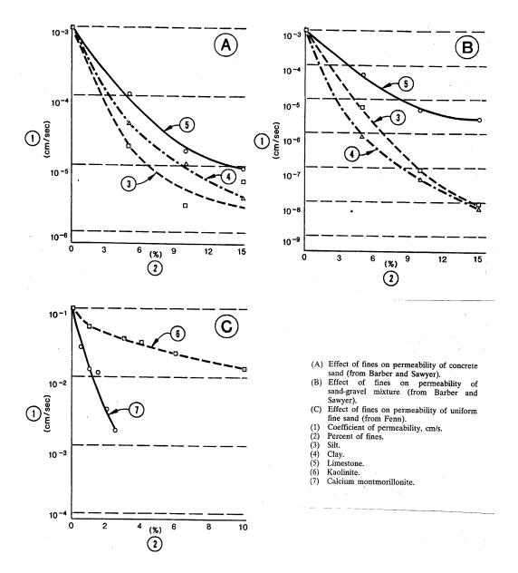
Figure 4 Influence of the type and amount of fines on permeability of concrete sand, sand-gravel mixture and uniform fine sand (ICOLD 1994 from US Army Corps of Engineers, 1986).
