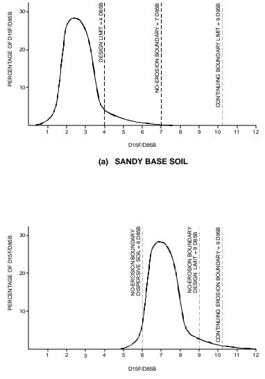
(b) FINE CLAY AND SILT, LITTLE OR NO SAND SIZED PARTICLES
