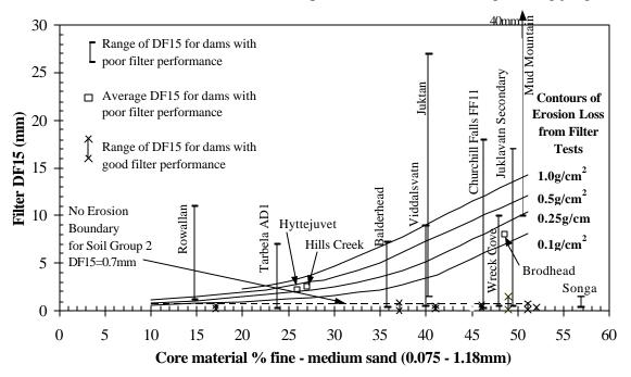
Figure 8 Comparison of erosion losses measured in filter tests to dams with poor and good filter performance (Foster and Fell 1999)
