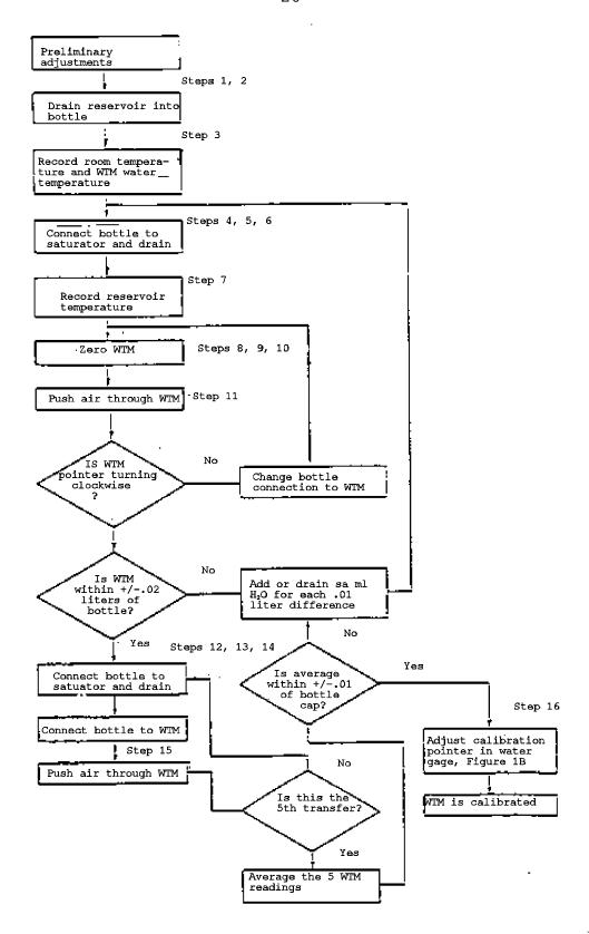
Figure 6. - Flow diagram for wet test meter calibration.
