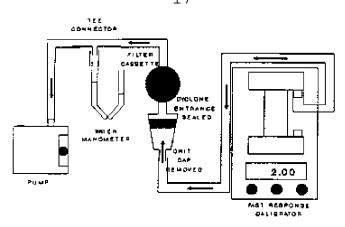
Figure 3. - Schematic showing fast response calibrator setup.
