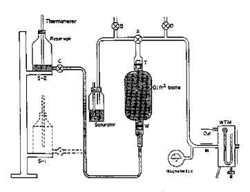
Figure 4. - Schematic showing equipment used for calibrating wet test meter.
