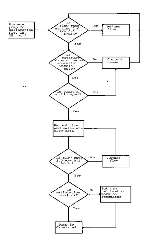
Figure 5. - Flow diagram for personal sampler calibration.
