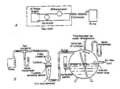
Figure 1. - Schematic showing  $(\underline{\mathtt{A}})$  Electrical circuit;  $(\underline{\mathtt{B}})$  calibration setup.
