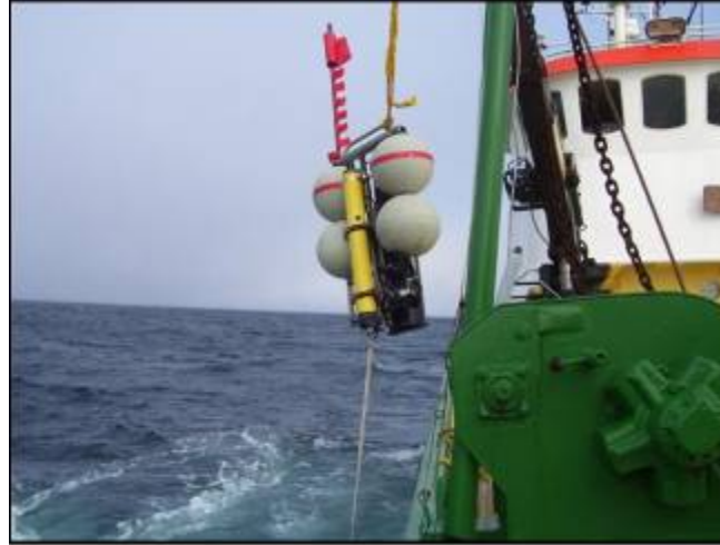
Figure 3: Ocean Bottom Hydrophone (OBH) recording system being deployed at sea. The OBH is a pop-up style autonomous recorder with very high recording resolution. Acoustic data is stored internally on hard-drive.
