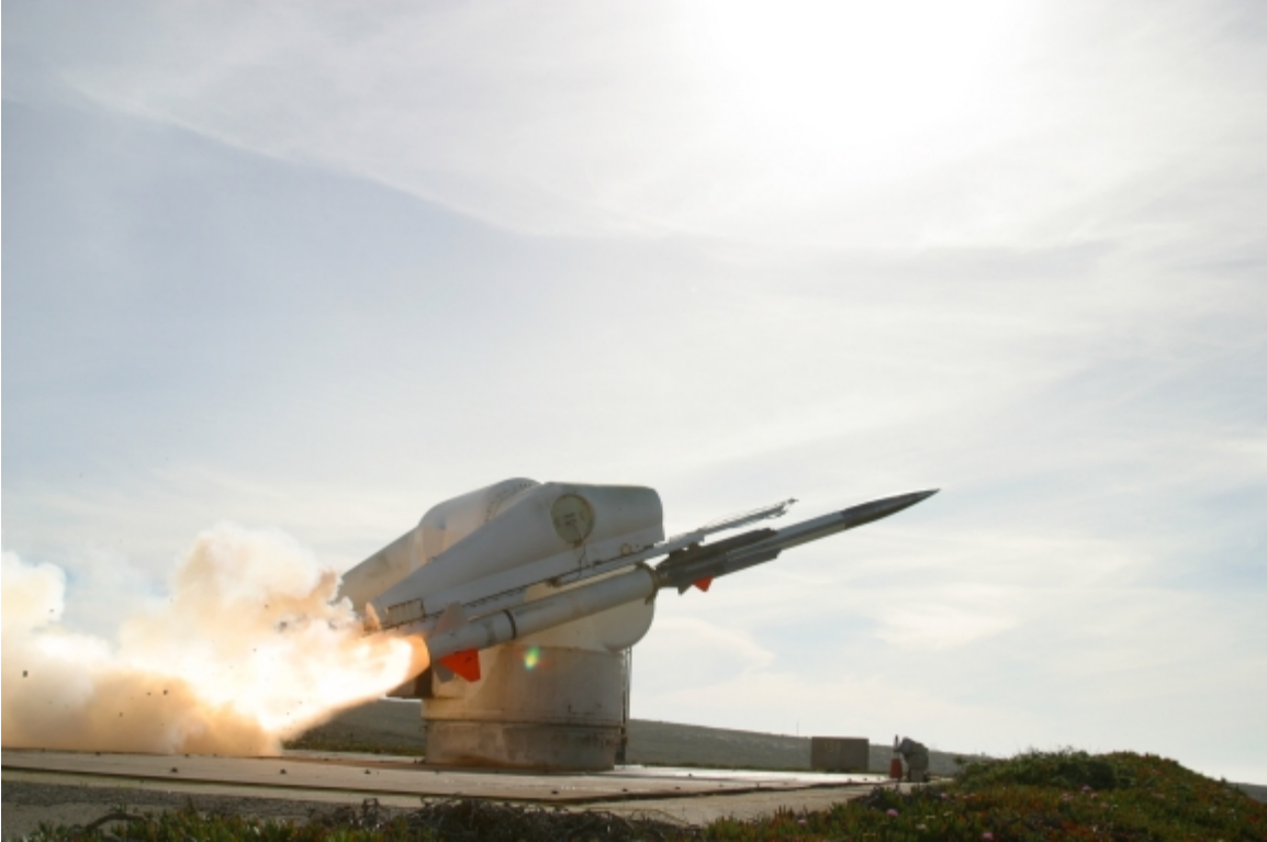
Figure 3. View of the Coyote with booster and launcher at the Alpha Launch Complex on SNI (photograph by U.S. Navy).
