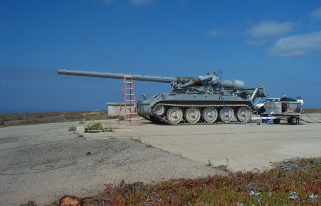
Figure 4. Howitzer used as AGS test launcher at the Alpha Complex (now located at the Building 807 Complex) on SNI (photograph by U.S. Navy).
