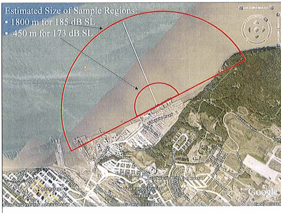
Projected sample area based on estimated transmission loss for 173 and 185 dB SL vibratory hammers
