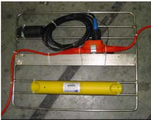
Single hydrophone group with acoustic transponder
