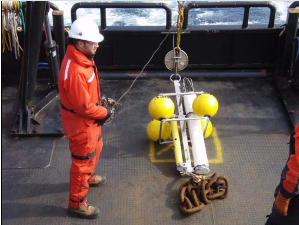
Figure 2. A picture of an ocean-bottom hydrophone (OBH) used to measure sound levels of vessels and seismic air guns.
