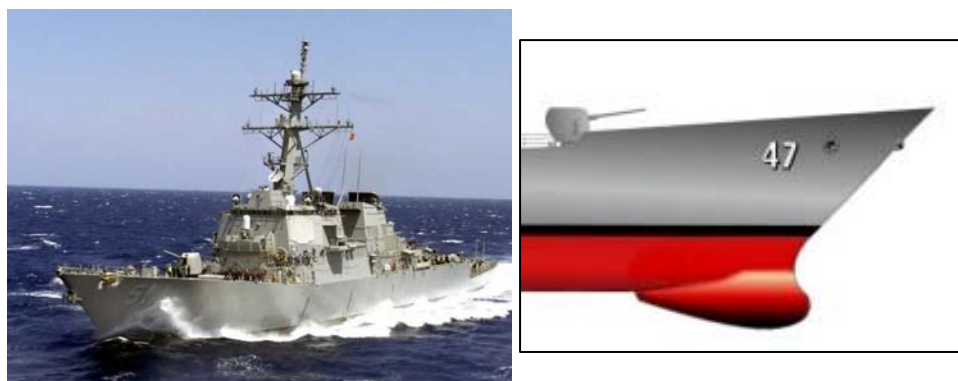
Figure C-1. Arleigh Burke Class DDG equipped with AN/SQS-53 (L); Ticonderoga Class CG showing AN/SQS-53 (R)
