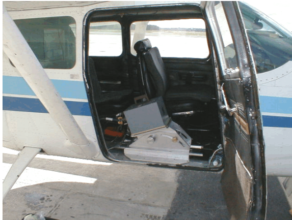
Figure 4.1. Example of variable-tilt sensor mount. One method of meeting the dual-look requirement is to fly the project area twice (once in each configuration) using a variable-tilt mount.
