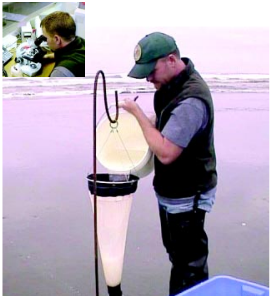
Above: ORHAB technician Anthony O'Dell collects plankton samples on a coastal beach. In the laboratory, (inset) he uses a microscope to identify and count HAB organisms in the samples.
