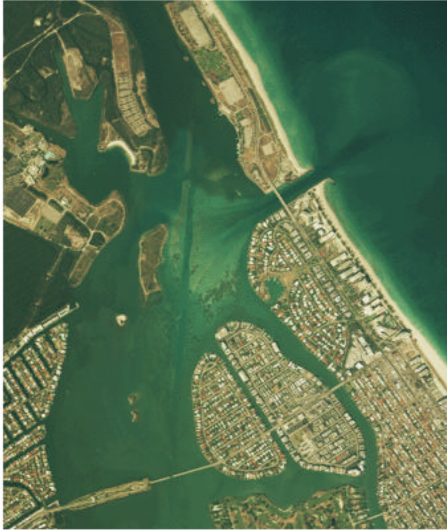
Figure 41. Bakers Haulover Cut. (The Oleta River is just off the image at the upper right. The Munisport Landfill site is almost directly east of Bakers Haulover Cut. Note sediment deltas on either side of the cut. Delta inside the Bay appears to have formed prior to dredging of the Intercoastal Waterway.) [Aerial photograph 5WPA1416, 1999. Scale 1:40000, azimuth 31.1, 25.88965° N, 80.16151° W. (Coastal Aerial Photography, NOAA/National Ocean Service, < http://mapfinder.nos.noaa.gov:80/mapfinderhtml3/surround/photos/photos.html >, < http://mfproducts.nos.noaa.gov/images/Photos/5WPA1416.gif >. See Figure 2 for identification details.]
