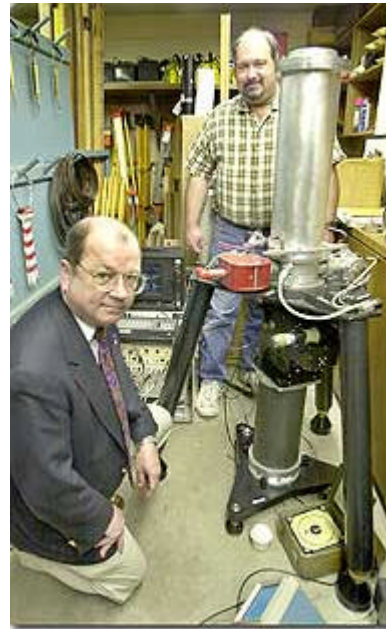
Advocate staff photo by Patrick Dennis LSU researcher Clifford Mugnier, left, and Daniel Winester of the National Geodetic Survey are using a gravity meter to measure tiny changes in elevation.
