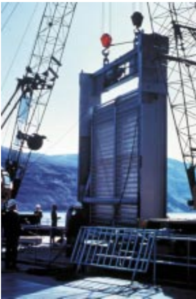
Submersible traveling screen at Lower Granite Dam for diversion of salmon smolts out of turbine intakes
