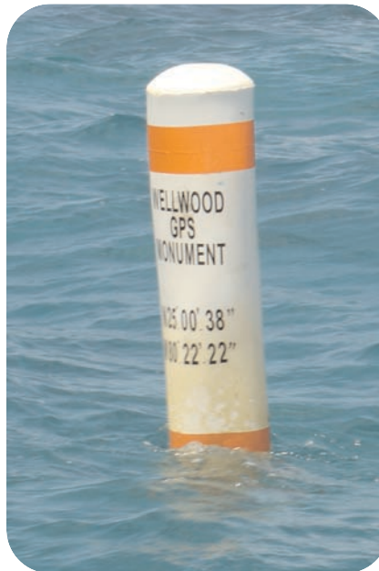
A spar buoy with the latitude and longitude marks the location of the geodetic marker placed on the seafloor. Boaters can use this marker to calibrate the accuracy of on-board navigational systems.
