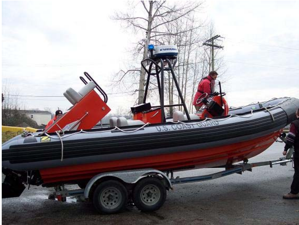
Cutter Boats - “Over the Horizon” rigid hull inflatables used for final stage interdiction.
