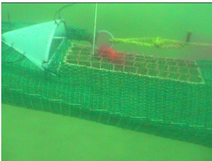
Figure 2. Square mesh panel with experimental fisheye BRD
