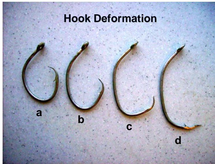
Figure 5: Examples of experimental hooks with varying degrees of deformation, (a) hook that landed a yellowfin with no bending evident, (b) yellowfin caught with minor deformation, (c) yellowfin caught with major deformation, (d) hook straightened, animal escaped.
