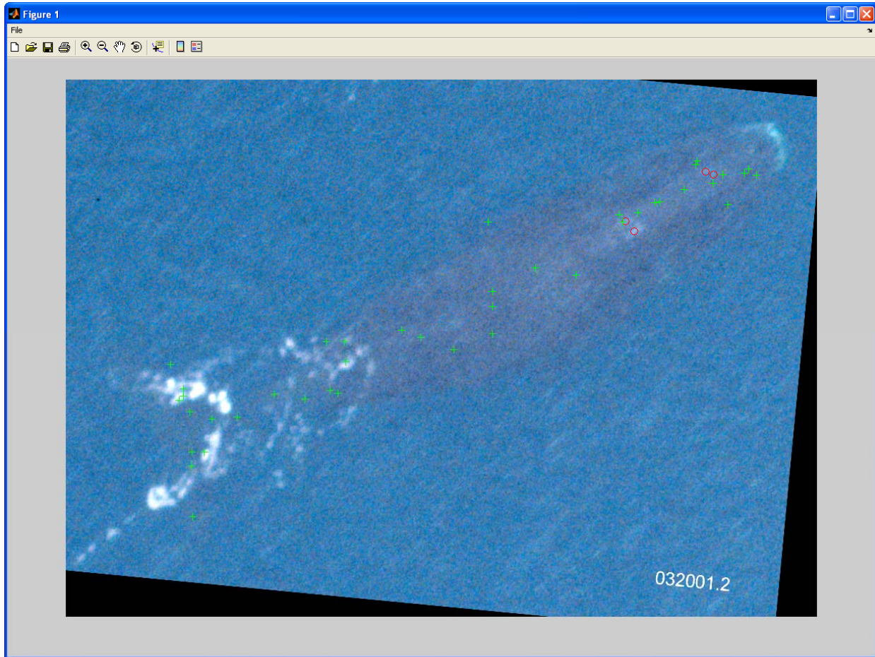
Fig. 20 - COMPARE TO LIST: From the window with the list of six images (Fig. 19), an image can be enlarged and compared to Image 1. When you click 'Enlarge', you can see the points from Image 1 overlapped on the enlarged image from the list. From this point, a trained technician will sort through all the possible matches to confirm if there are true matches.
