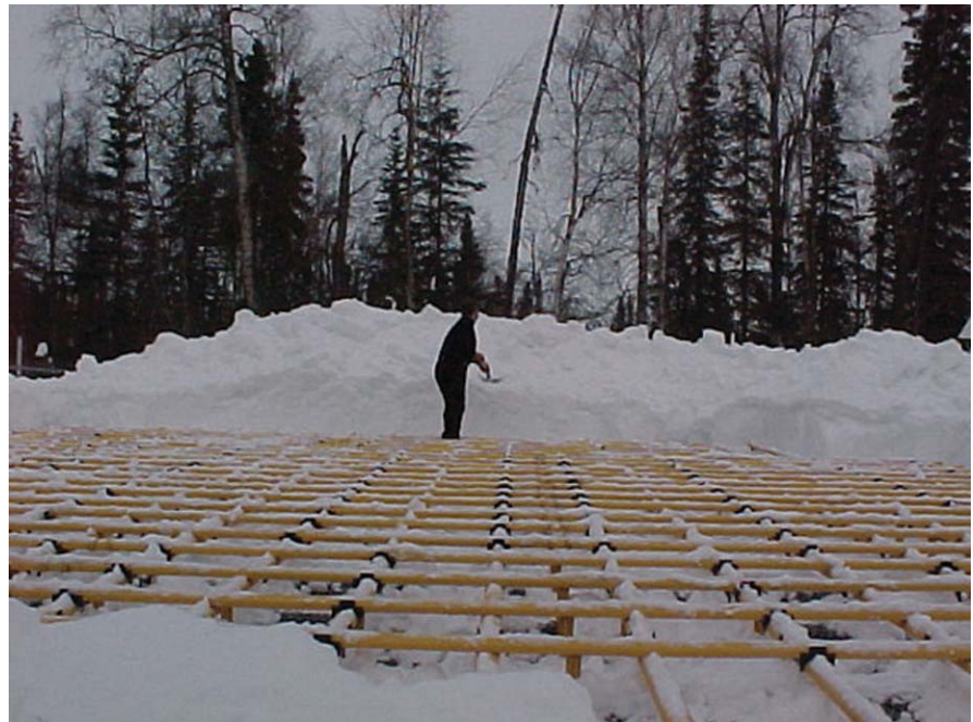
Figure 53. National Weather Service technician removing snow from the profiler antenna at Talkeetna, Alaska.
