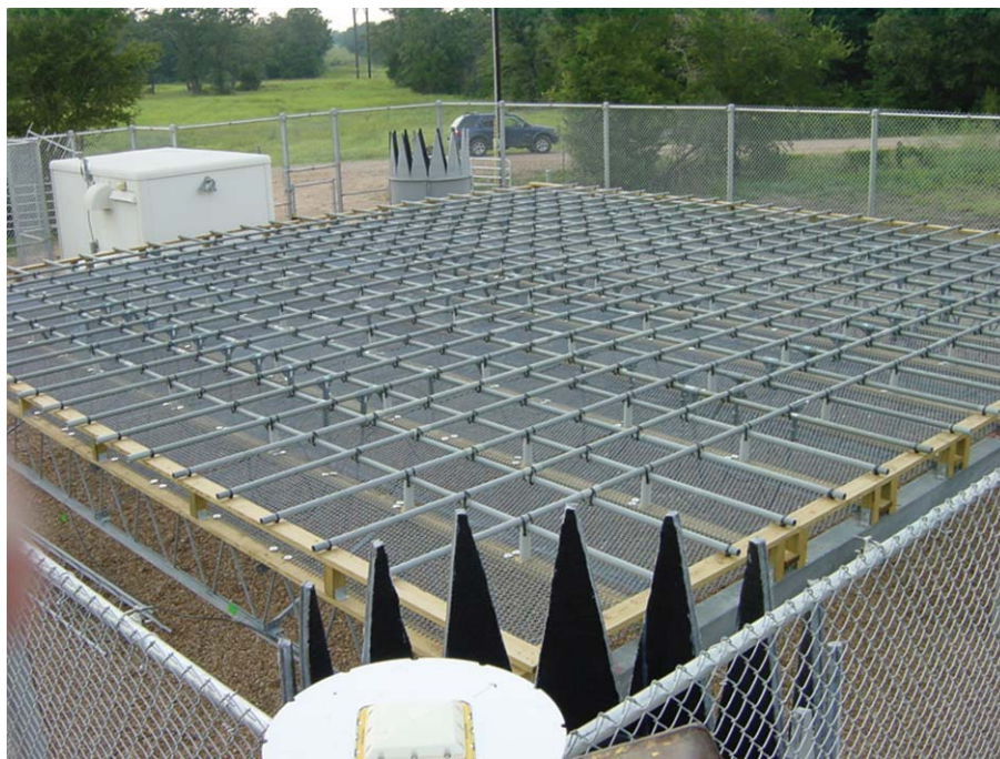
Figure 49. Profiler located at Ledbetter, Texas: antenna (horizontal grid), equipment shelter containing all electronic components (upper left), RASS temperature profiling components (crown-like instruments), and GPS-Met Integrated Water Vapor Monitoring system (bottom center).
