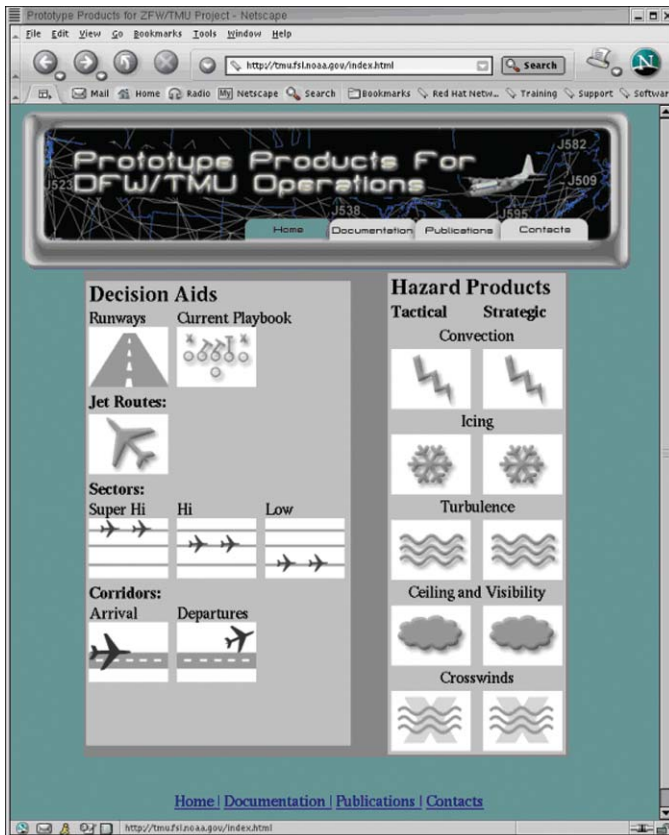
Figure 74 . Screen from the TMU Website showing icons that traffic managers can click to see the actual weather hazard.
