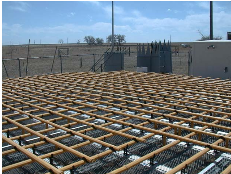
Figure 52. The 449-MHz profiler at Platteville, Colorado, planned as a testbed site for a national 449-MHz profiler network. (Photo courtesy of Brian Koonsvitsky, SRG Inc.)
