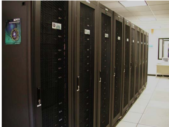
Figure 8. An example of newly installed equipment (280 Alpha CPUs and 1536 Pentium IV-Xeon CPUs) in the Phase III upgrade of FSL's High-Performance Computing System.
