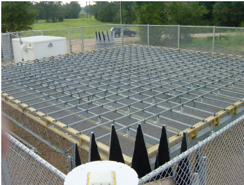
Figure 51. The 404-MHz profiler at the Lower Colorado River Authority's Natural Science Laboratory in Ledbetter, Texas. (Photo courtesy of Brian Phillips, SRG, Inc.)
