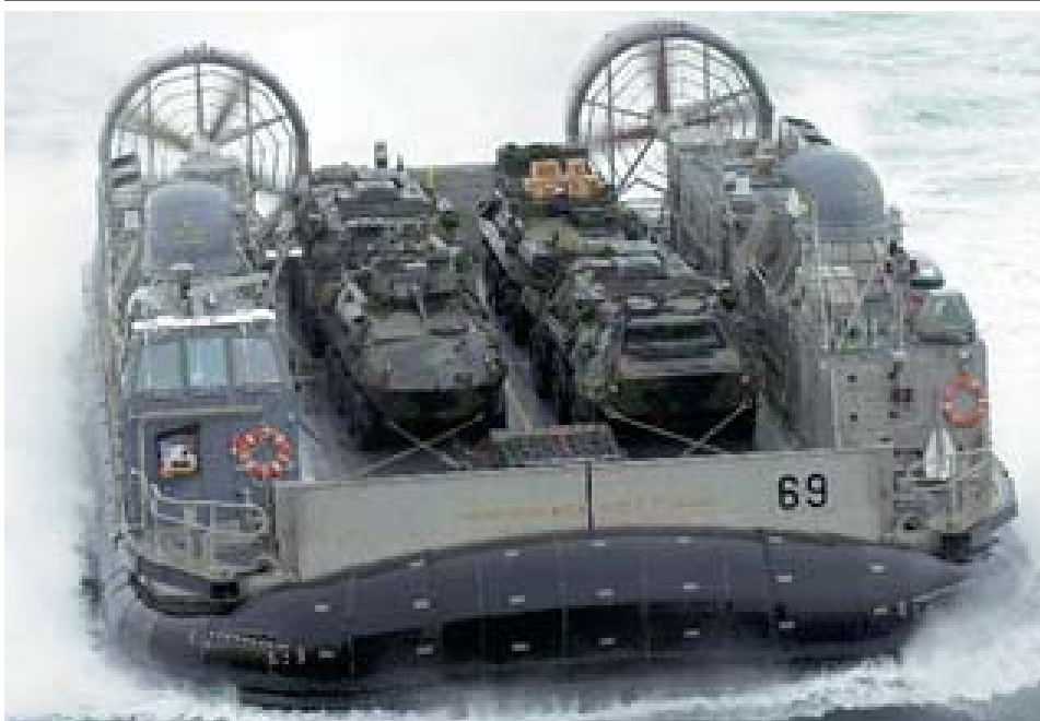
Figure 3-DOD-14. A Landing Craft Air Cushion (LCAC) Vehicle from Assault Craft Unit Four (ACU-4) transports Marine Assault Vehicles to the USS KEARSARGE (LHD 3). (US Navy Released)
