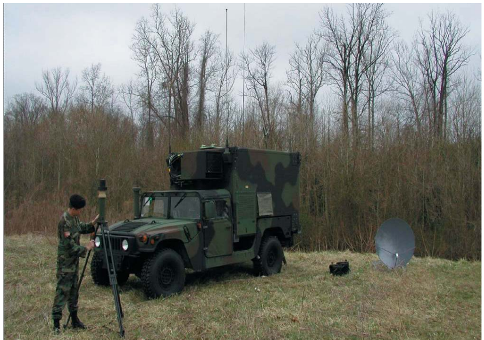
Figure 3-DOD-23. Meteorological Measuring Set- Profiler (MMS-P) obtains upper level wind data for artillery fires. (U.S. Army Released)
