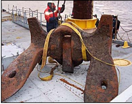
Figure 2. Submerged objects recovered from the vicinity of the Athos grounding location.
