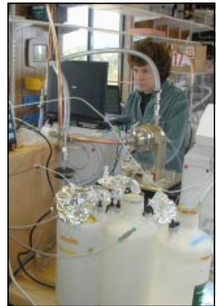
Tim Bates/NOAA Theresa Miller of NOAA's Pacific Marine Environmental Laboratory adjusts an instrument in one of two hilltop trailers that measures the water soluble inorganic component of aerosols in the atmosphere.
