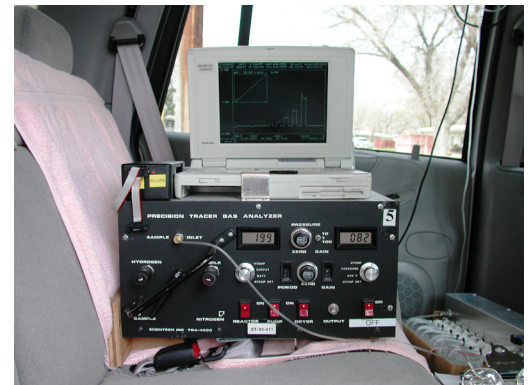
A fast response analyzer that measures tracer concentrations every second. The analyzer is easily carried in the back seat of a vehicle. Photo: NOAA/ARL
