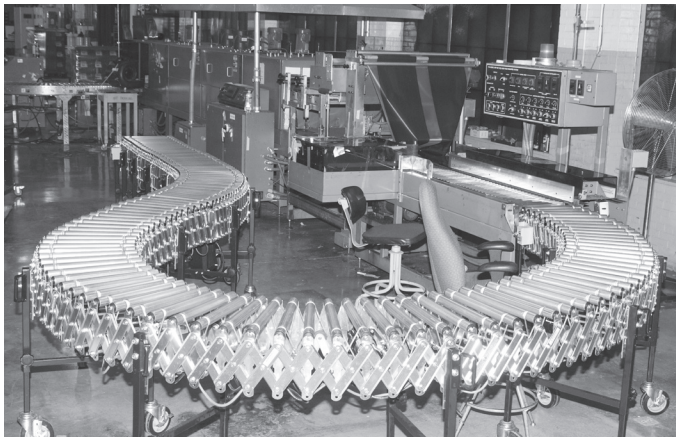
The new conveyor system attached to the note packaging machine will package currency more efficiently, while reducing injuries caused by repetitive lifting.
