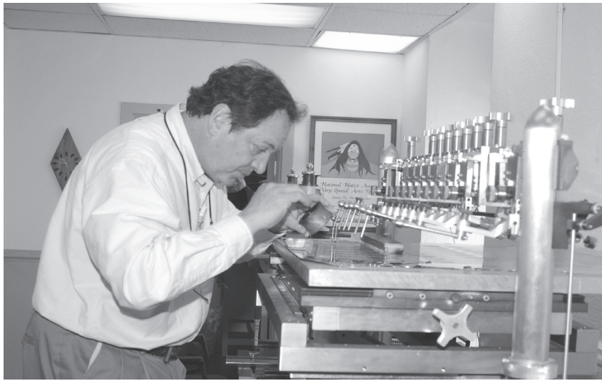
Gary Slaght, Engraver, numbers an engraved plate manually. The manual pantograph is used to etch the same image into multiple locations on a plate.
