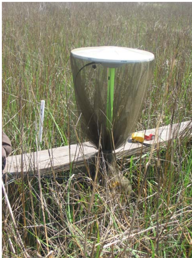
Figure 9. GNSS antenna deployed atop a Surface Elevation Table (SET) bench mark, covered with a double layer of mosquito netting for camouflage.
