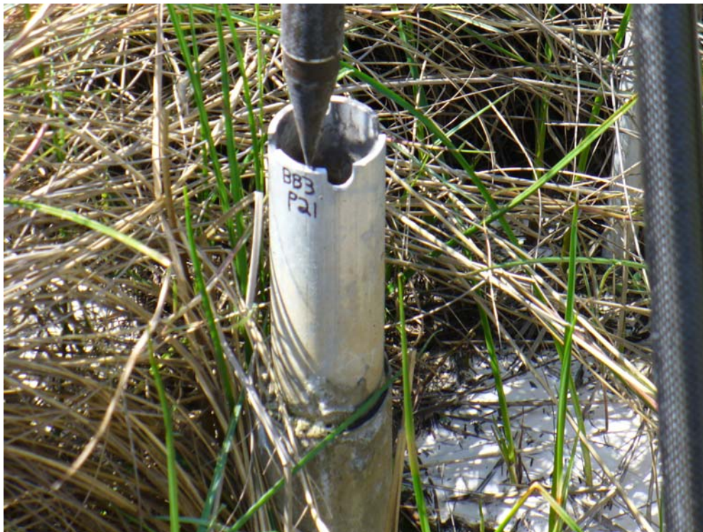
Figure 2.1. Surface Elevation Table (SET) bench mark (BM) top type #1 (of 3): A 2-inch diameter aluminum pipe with four predetermined positions (notches) for the SET. Shown is an RTK GNSS survey underway. A dimple marks the Vertical Point of Reference (VPR), the highest point on the BM.
