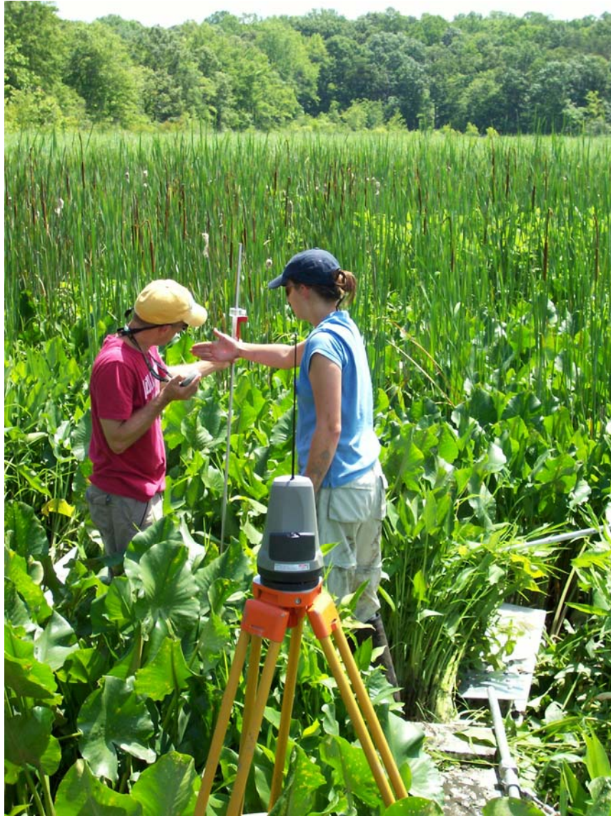
Figure C.6. The RoboLaser™ technique in operation in a tidal freshwater wetland. The remotely operated, self-leveling level is shown in the foreground. The operator, on the left, is holding the remote control used to direct the laser beam horizontally. A customized level rod slider is used to help keep the level rod plumb while adjusting the level and reading the height off the rod.
