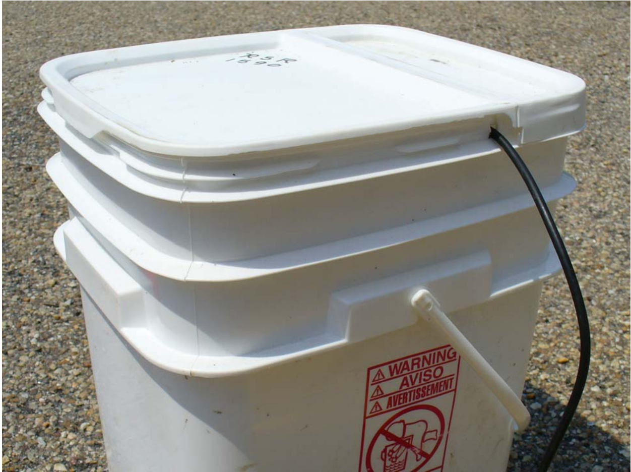
Figure 8.2. Notch cut in top edge of bucket to allow for GNSS antenna cable.
