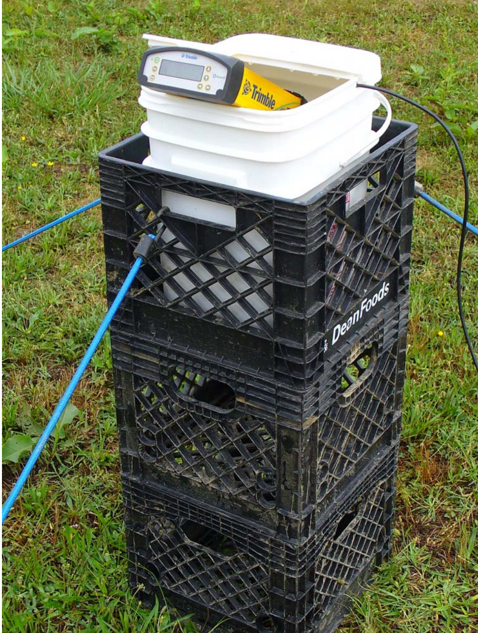
Figure 8.1 GNSS-in-a-bucket (lid open), cost-effective method to keep receiver high and dry.
