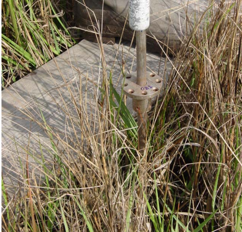
Figure 2.2. SET BM top type #2 (of 3): A 9/16-inch stainless steel rod w/eight-hole collar for orienting the SET. A leveling staff is being backsighted in the determination of the height of a GNSS antenna (or SET) above the BM.
