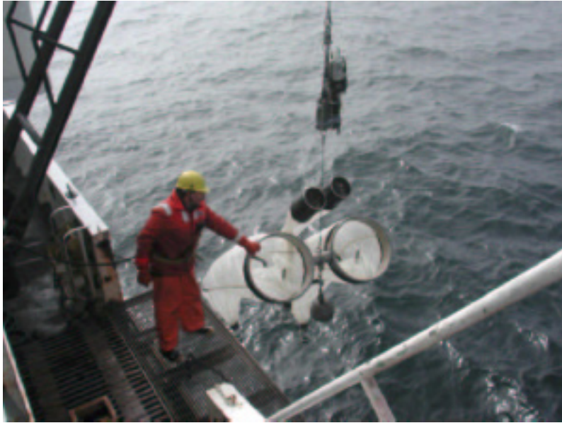
A bongo net with Seacat instrumentation being deployed for fish-larval studies.
