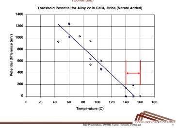
This figure is an overhead from Dr. Farmer's presentation at the May 13, 2003, Board meeting in Washington, D.C. Note the dashed boxes. They indicate that base-metal steady-state corrosion potential moves in a noble (positive) direction with time and that welded-metal corrosion potential moves even farther in that direction with time, indicating increasing susceptibility to crevice corrosion with aging time and in welded structures. Although the overhead appears to state that
