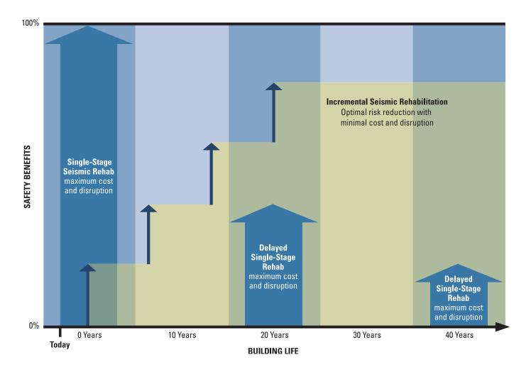
Incremental Seismic Rehabilitation Element 9 **Budget Packaging**  Incremental seismic rehabilitation affords great flexibility in the sequence and timing of actions when the following precautions are kept in mind:
