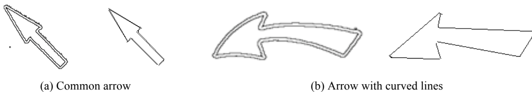
Figure 5. Results of line segment approximation of symbol boundary. Boundary on left of each subfigure is the original boundary and the one on the right is the line-segment approximated boundary.
