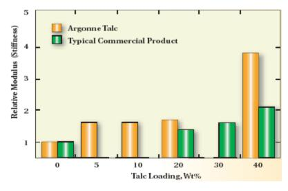
The data in the bar chart show the effect of compounding the first-generation Argonne-modified talc into polypropylene. With only 5 wt% mineral loading, the modulus is increased by 62%. This compares favorably with conventional talc-filled polypropylene, which generally produces a more modest increase in modulus of 30–40%, but requires four times the mineral loading. At the highest loading levels, the Argonne materials are almost twice as stiff as conventional talc-filled polypropylene.
