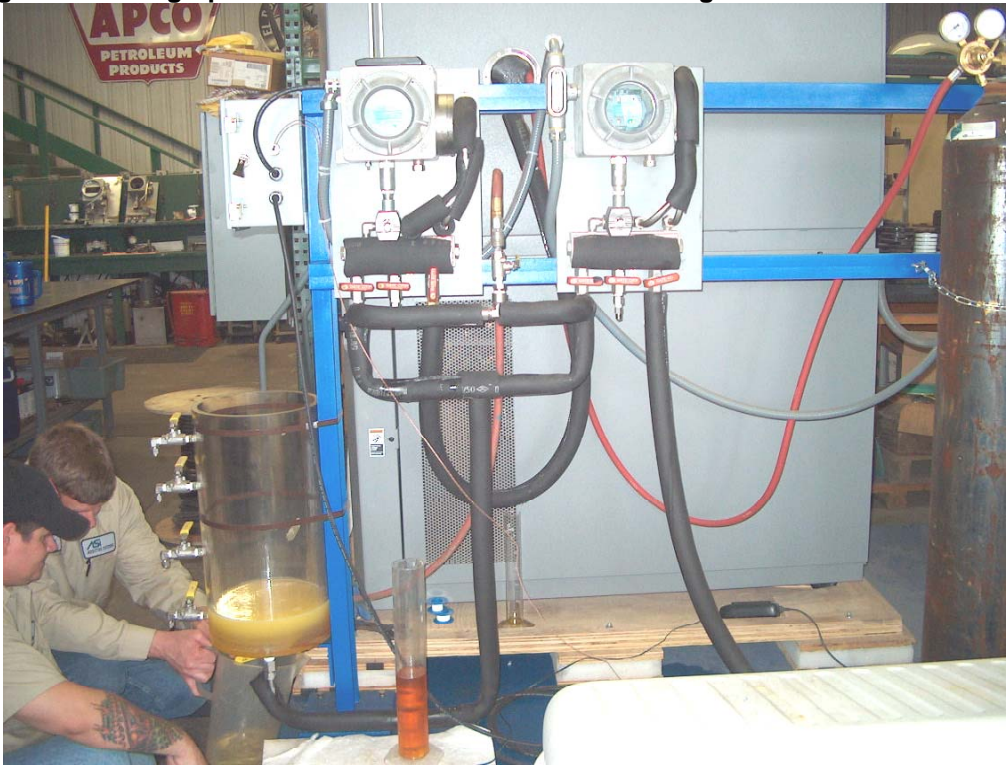
Figure 1. Photograph of Small Scale Test Unit for Blending Biodiesel and Diesel Fuel
