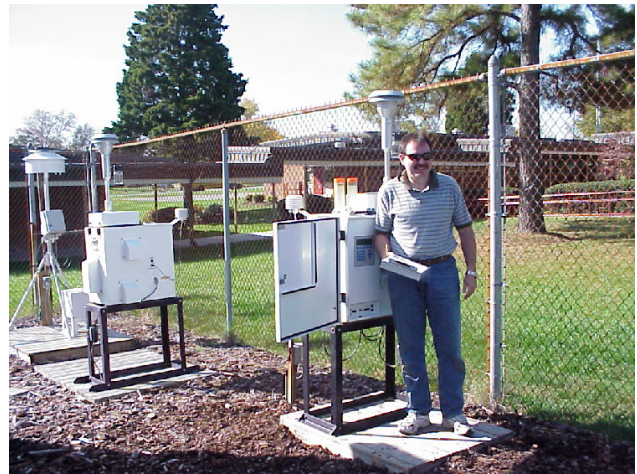
DEQ's Anton Sorkin installs a particle pollution monitor at a Henrico County site.
