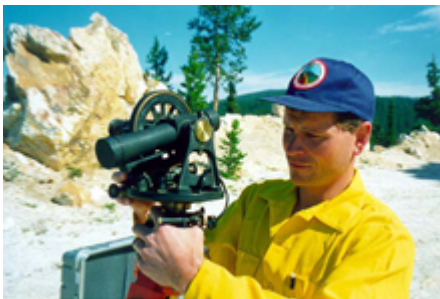
NOAA forecaster Troy Lindquist of the NOAA National Weather Service forecast office in Grand Junction, Colorado, uses a theodolite to align the angle a weather balloon takes after being launched.
