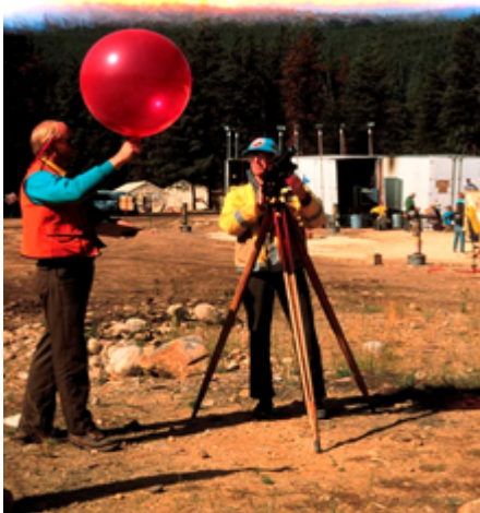
IMET Carl Gorski prepares to track a Pilot Balloon (PIBAL) at a fire incident as a Fire Behavior Analyst prepares to launch the PIBAL.
