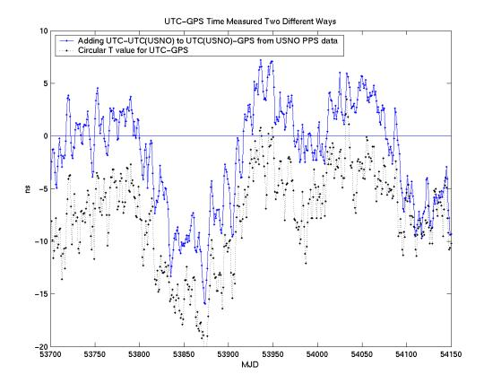
Figure 8. UTC-GPS as reported in the Circular T, and UTC-GPS inferred by subtracting UTC (USNO) – GPS from UTC – UTC (USNO). UTC (USNO) – GPS can be obtained from the satellite broadcasts, as in Figure 5 and is also measured directly at the USNO.
