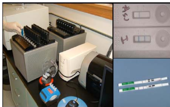
Figure 2: Molecular diagnostic equipment (left) Device used for DNA analysis to identify plant pathogens and pests in several stages of development (right) Antibody-based tests suitable for field deployment to test for plant pathogens
