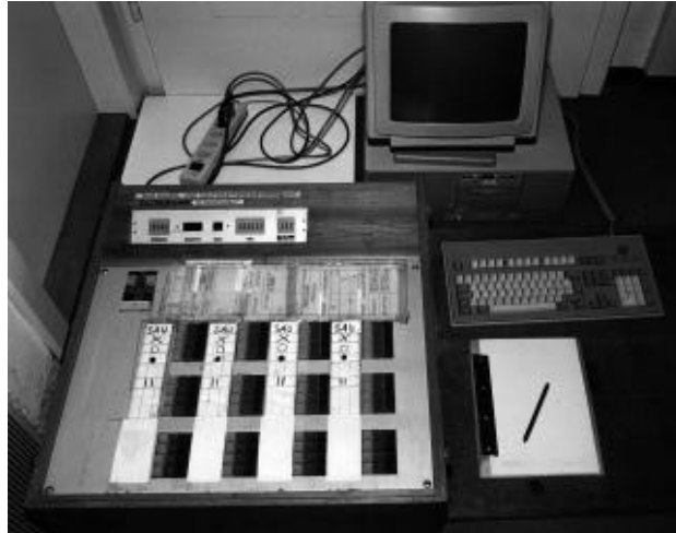
Figure 4: Electronic device to register time and frequency of animal- behaviour in quantitative terms
